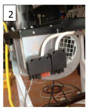
Disconnect the gas pipe from the valve group to the burner body.....
