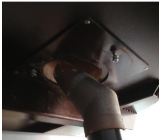
Insert the burner through the oven hole and the 3 holes with screws
