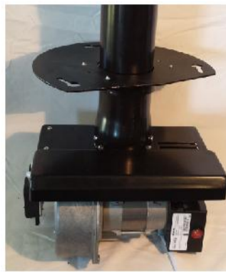
Burner prepared in-place with flange
