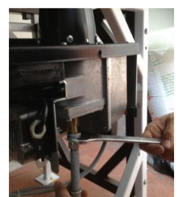
Connect the tube with the burner body
