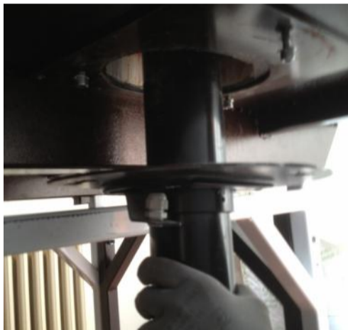
Insert the burner through the oven hole and the 3 holes with screws
