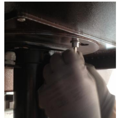
Turn the burner 15 degrees following the holes and lock the 3 screws
