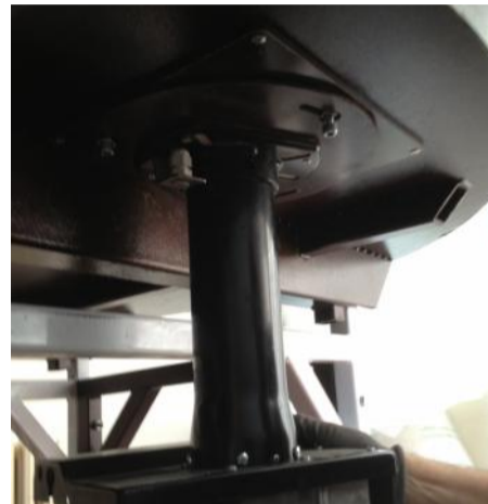
Turn the burner 15 degrees following the holes and lock the 3 screws
