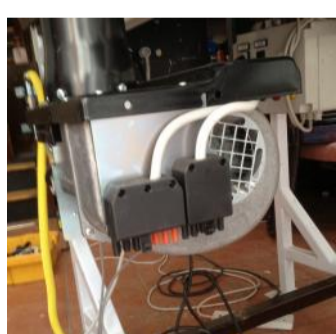
Connect the multi-polar connectors of the switchgear and the valve group to the burner
